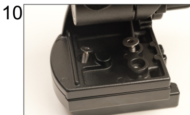
Insert screw into original head. Smaller screw goes into opening near to round surface
