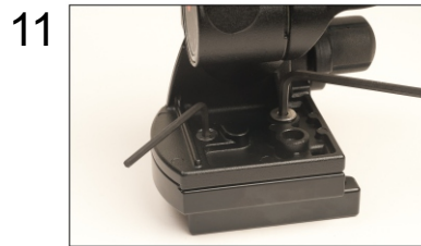
Attach conversion plate to original head with two screws
